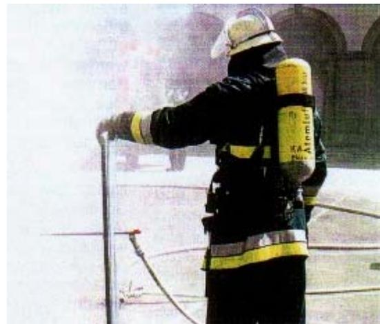
The hole can be made with the included hammer or using a drill with a diameter of 17,5 mm or more. Thin materials such as wooden doors or car tin can be perforated with the nail being driven in by the hammer. There are two kinds of Fognails that can be distinguished by their spraying patterns (*exhibit 1*). The spraying pattern is determined by the layout of the nozzle’s holes (*pictures 2 and 3*).
