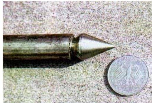
Fognail "Restrictor" is used preferably to build a blockade. It can also be applied to confine heat and lower the temperatures in the area of fire. It is not suitable for a targeted spraying of extinguishing agent onto the seat of fire (*picture 4*).
