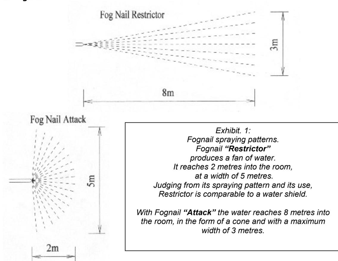
Fognail is a kind of extinguishing lance at the tip of which finely dispersed water emerges. Water is provided through a D-hose and the common centrifugal pump of the vehicle. The manufacturer claims a water use of 70 litres per minute at 8 bar. The nail is brought to the area of fire through a prepared hole (*picture 1*).
