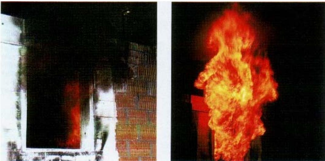
After 17 minutes, 40 percent of all combustible material is burnt, the fire is fully developed. The command is given to fight the fire while the door is closed – using Fognail.
