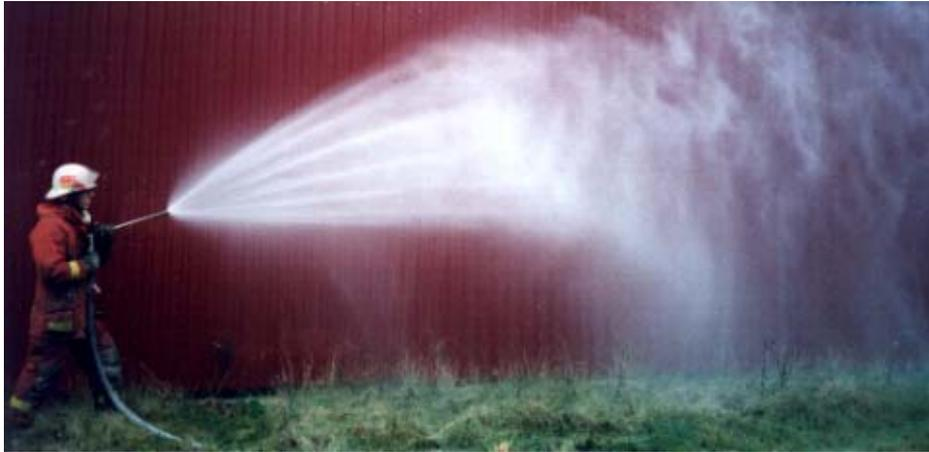
According to the manufacturer, FogNail's extinguishing effect is based on two factors: the cooling effect of the water and the oxygen-extinguishing effect of the immediately generated water vapour.
